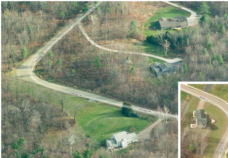
Above: This road is more suited to a rural subdivision. It is relatively narrow and gravel surfaced, and some sections are tree-lined. It provides adequate access for emergency and service vehicles but is not overbuilt.
