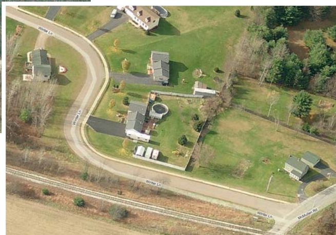
Above: This road is more suited to a rural subdivision. It is relatively narrow and gravel surfaced, and some sections are tree-lined. It provides adequate access for emergency and service vehicles but is not overbuilt.
